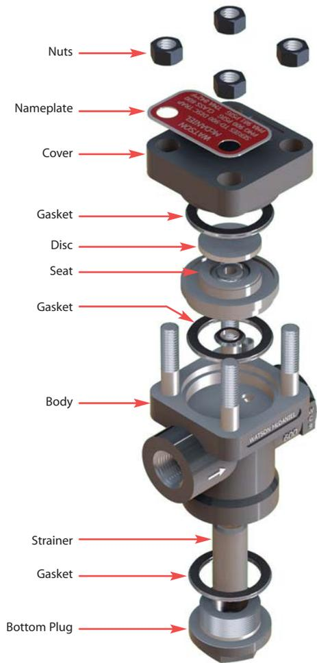
Complete internal working mechanism can be replaced while trap body remains connected in-line
