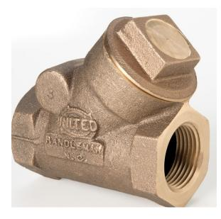
Model 62 Swing Check Valve Complies with MSS-SP-80-2013 CRN OCO7135.2C 200WSP @ 406° Max 400 WOG 100% Pressure Tested Threaded Ends \*Contains Lead. Not Intended for Use in Potable Water Systems\* Install in horizontal position with cap in upright position. Not recommended for pulsating or vibrating service.
