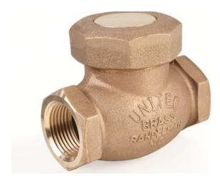
Model 50T Check Valve Spring Loaded Lift Check Complies with MSS-SP-80-2013 CRN OCO7135.2C 200WSP @ 406° Max 400 WOG 100% Pressure Tested Threaded Ends • PTFE Disc Integral Seat \*Contains Lead. Not Intended for Use in Potable Water Systems\*
